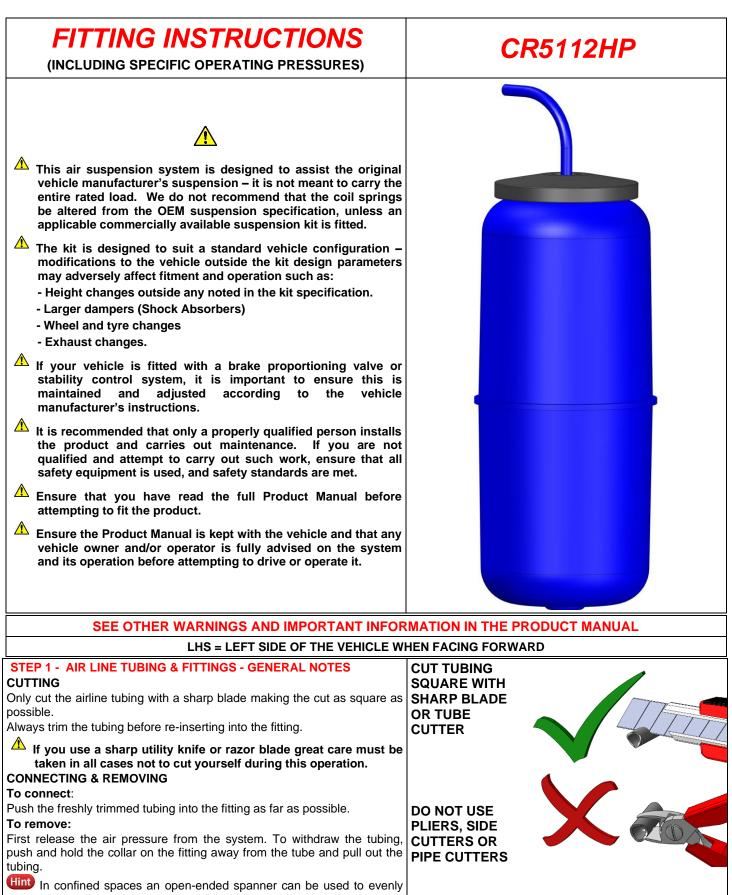
depress the collar and remove the airline tubing.
